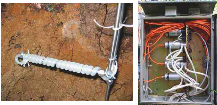
Figure 2. Gas collector installation in the soil (on the left) and the installation box for the GMP343 probes (on the right).
