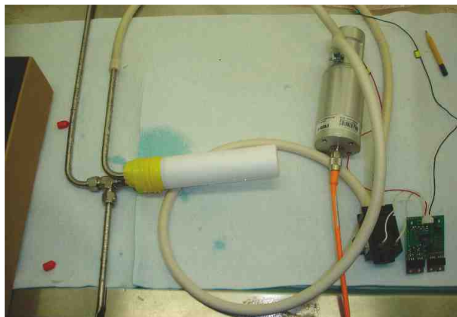
Figure 3. Test installation with a sintered PTFE chamber.
